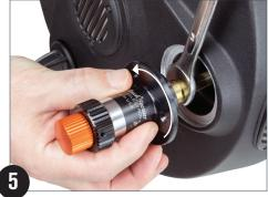
Use the crescent wrench to hold the brass bushing stationary while rotating the body of the FeatherTouch MicroFocuser counterclockwise until it unthreads and detaches from the brass bushing.
