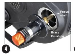
Pull out the FeatherTouch MicroFocuser so that the brass bushing on the focus shaft is exposed and accessible.
