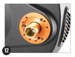
Locate the cover plate for 11" and 14" telescopes included with the Celestron Focus Motor and install it onto the RASA 11 using the 3x screws from step 3 above. Orient the cover plate as shown.
