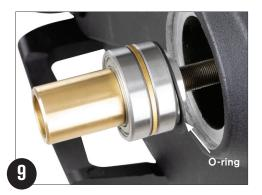
Thread the Celestron focuser onto the focus shaft several turns, make sure the O-ring is still resting on the nut on the focuser and not the focus shaft.
