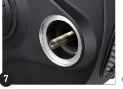
Unthread and remove the brass bushing
