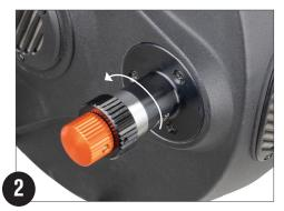
Rotate the black focusing knob of the FeatherTouch MicroFocuser counter-clockwise as far as it will go.
