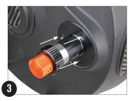
Remove the 3x screws that connect the FeatherTouch MicroFocuser to the RASA 11. Save the screws; they will be used later to install the focuser cover plate that comes with the Celestron Focus Motor.
