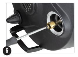
Unthread and remove the screw and washer from the end of the focus shaft.
