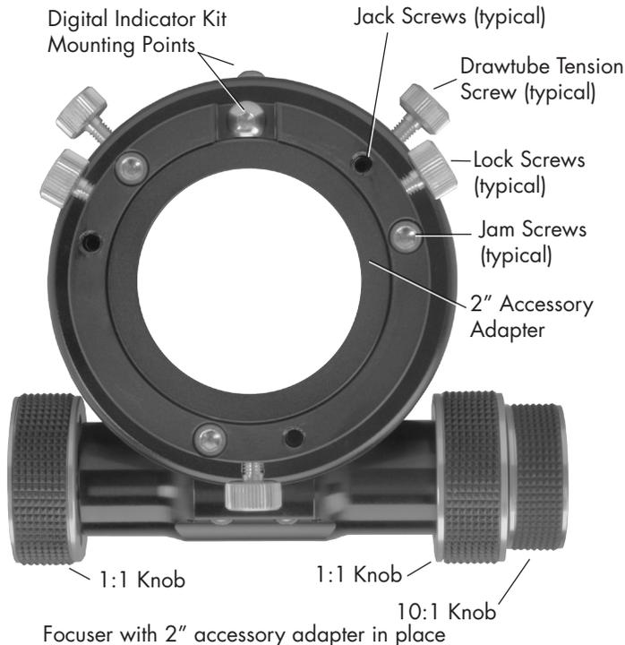
The two tension screws on the top of the focuser body can be adjusted to add resistance when using heavy equipment. These tension screws tighten against a brass clamp ring, which then cinches down on the Teflon sleeve in which the draw tube slides. For photography it is not necessary to tighten beyond the need to keep a camera stationary but we do recommend to tighten them in unison to avoid any focus shift. Note that even when sufficiently tight, the focuser knobs can still drive the draw tube.
