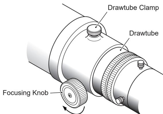
Drawtube will move out of the telescope tube by turning the focusing knob clockwise.
