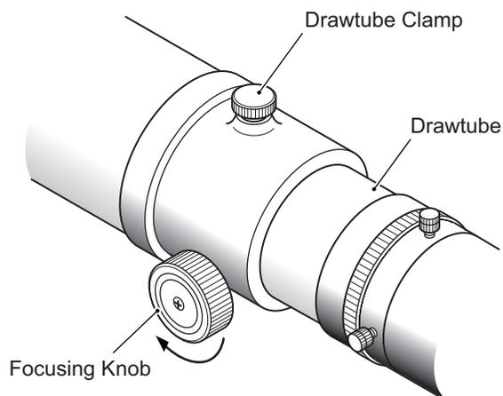
Drawtube will be moved out by turning the knob this direction.
