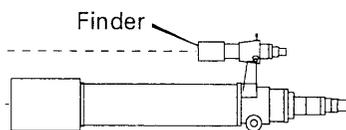
Before placing the finder into the finder holder, wrap three layers of clear cellophane tape around the tube of the finder where the front set screws make contact with the finder. The rear set screws have a protective nylon cover over the end of the screws to prevent them from scratching the tube.
